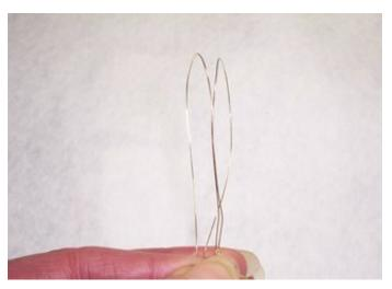
This is the cool part...no more need for a drawing to make identical left and right wing. Loop both wires over your finger and back down to the top of the twisted wires. You now have identical shapes.
