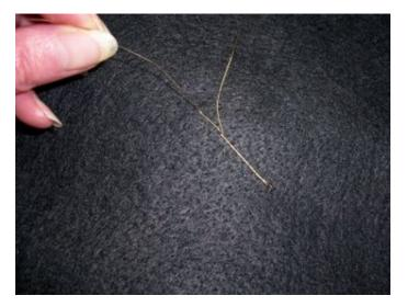
Twist the bottom approximately 1" up the length of the wire.
